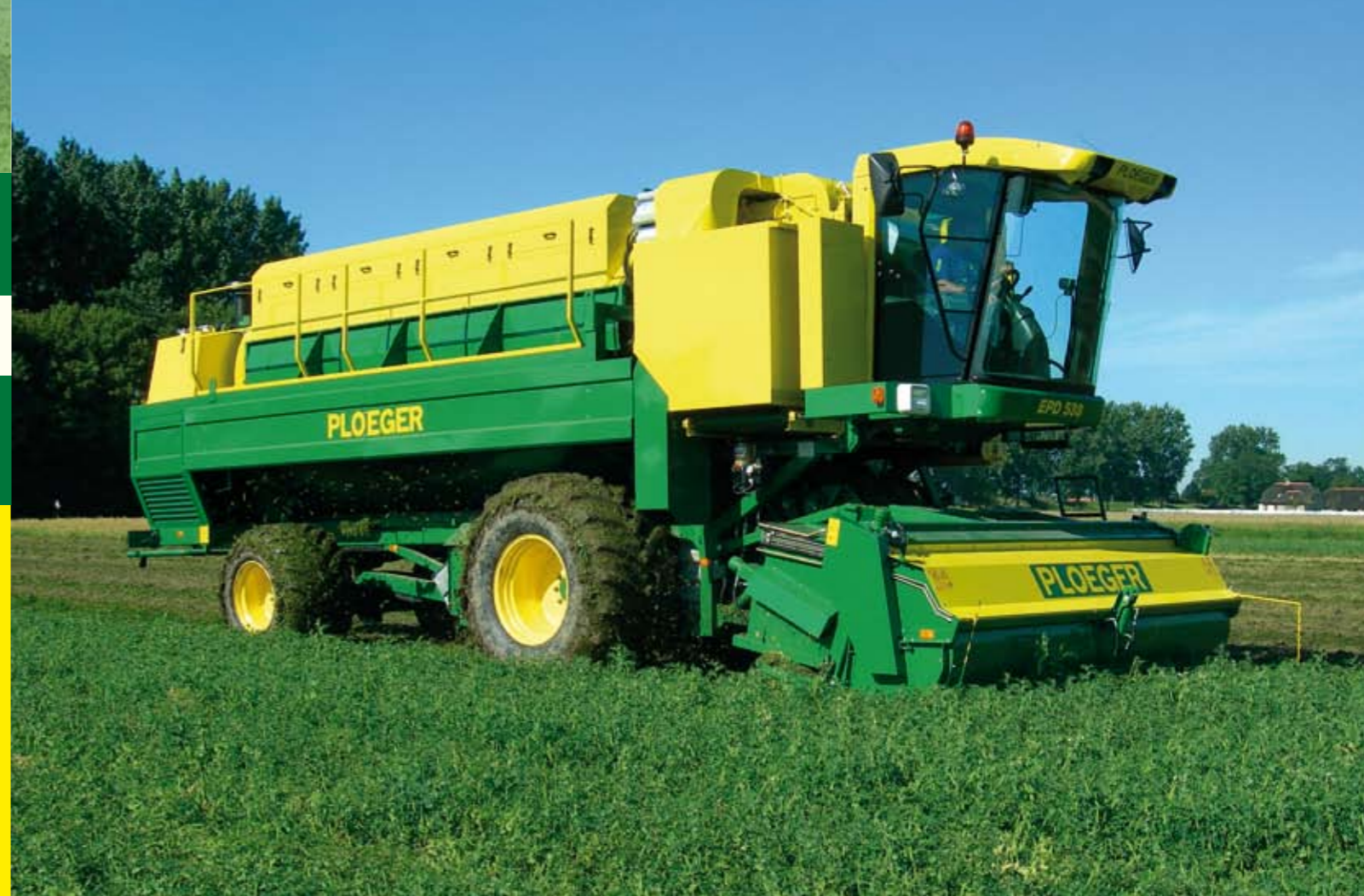
4 630 mm wide tracks and 5 meter new model picking head
