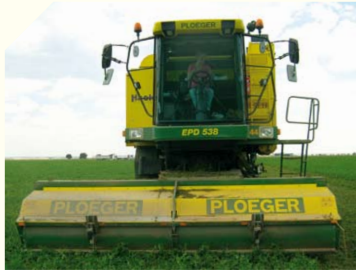
3 EPD 538 with a 5 meter wide new model picking head w/o ground roller
