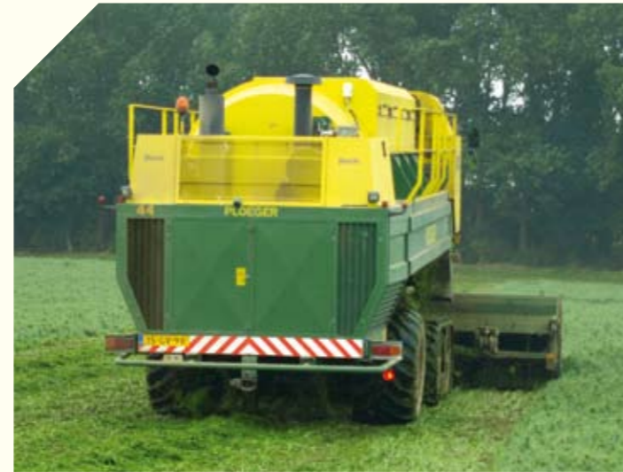
4 630 mm wide tracks and 5 meter new model picking head
