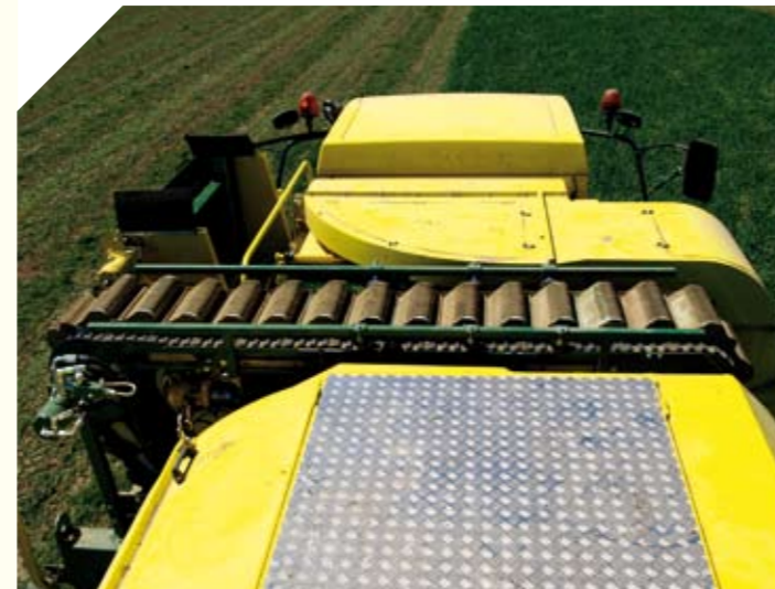
1 New model bigger volume bucket elevator, with a 34% increased top cleaning system
